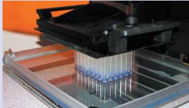
simplified version! The Perfactory® system works like a copy station. It builds solid 3D objects by using the DLP® projector to project sequential voxel planes into liquid resin, which then causes the resin to cure from liquid to solid. Each voxel plane made up of tiny Voxels (volume pixels), with dimensions as small as  $16\text{ }\mu\text{m} \times 16\text{ }\mu\text{m} \times 15\text{ }\mu\text{m}$  in X, Y and Z direction. It's like building your part from very small Lego blocks!
