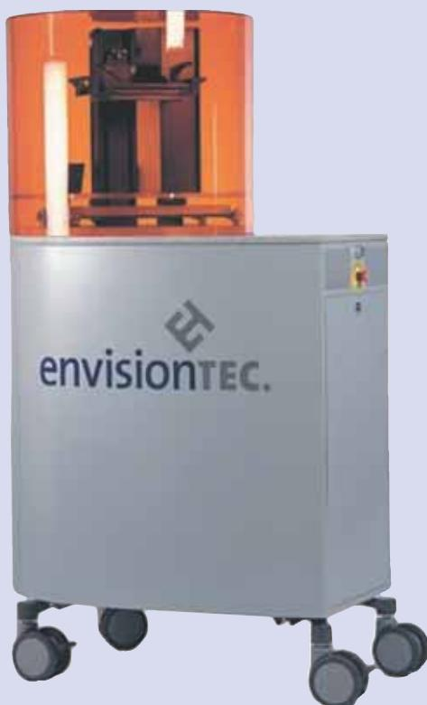
direction) with a dynamic voxel thickness from 25 µm to 150 µm and a build speed up to 20 mm per hour.
