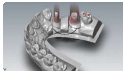
Fig.4 Insertion axis modification in CAD
